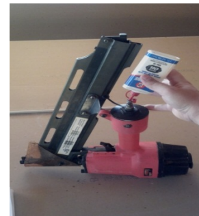
Figure 7 - Insertion of oil into nailer
